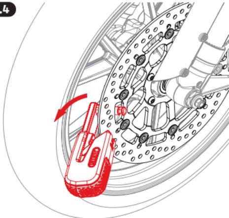
**8.1** Closing without a brake disc (transport mode)
