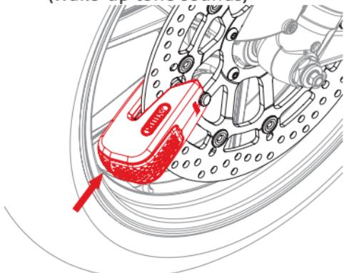
**7.3** Pull the lock body away from the brake disc using light force, the lock opens automatically
